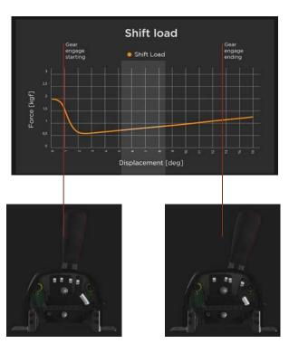
In the **initial phase** of operation, the shift lever exhibits greater resistance, simulating the movement of the shift mechanism.
